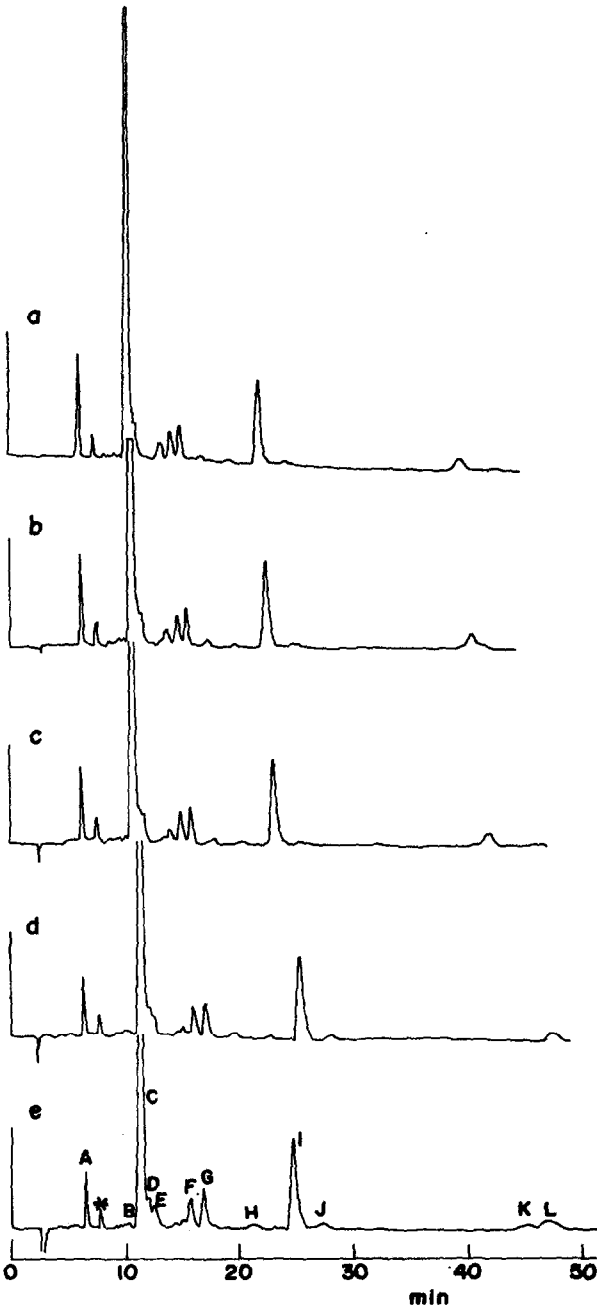
Fig. 1. Analytical chromatograms of urushiol in the sap of Rhus vernicifera from Hupei, China. Conditions: column, Develosil ODS-5 ( 5\ \mu\text{m} ), 25 \times 0.45\ \text{cm} I.D.; flow-rate, 1.25\ \text{ml/min} ; detector, 254\ \text{nm} , 0.32\ \text{a.u.f.s.} ; eluent, acetonitrile-water-acetic acid (90:10:2) containing silver nitrate: (a) 5.8, (b) 11.6, (c) 29, (d) 58 and (e) 116 mM.
